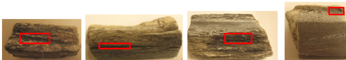
Figure 6 From left to right, samples 4, 3, 2, 1. The red squares are where samples were collected for Carbon 13 isotopes.
