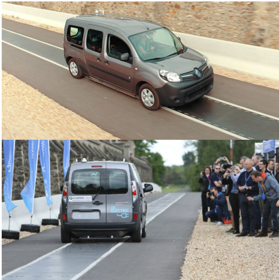
Figure 1.1: Qualcomm and Renault testing dynamic wireless charging in France. Adopted from [28, 50]
