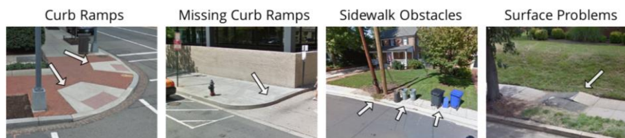
Fig. 1. Example of Problem Sidewalks and how they are labeled in “Project Sidewalk” [16]
