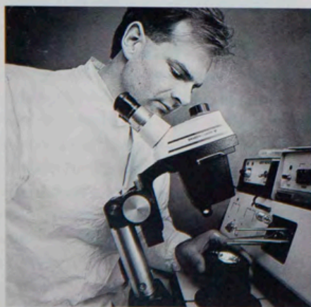
In the Electrical Engineering laboratory, a student uses an ultrasonic bonder to attach wires, smaller in diameter than a hair, to contact pads on an integrated circuit (IC) chip for characterization.
