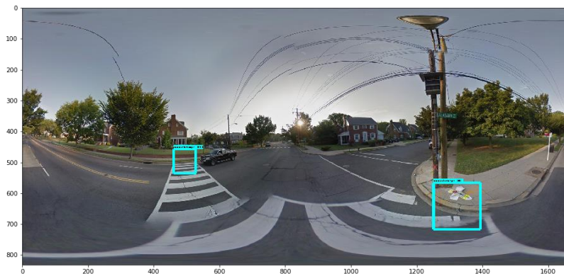
Figure 2. Example model output showing correct detection of missing curb ramps.
