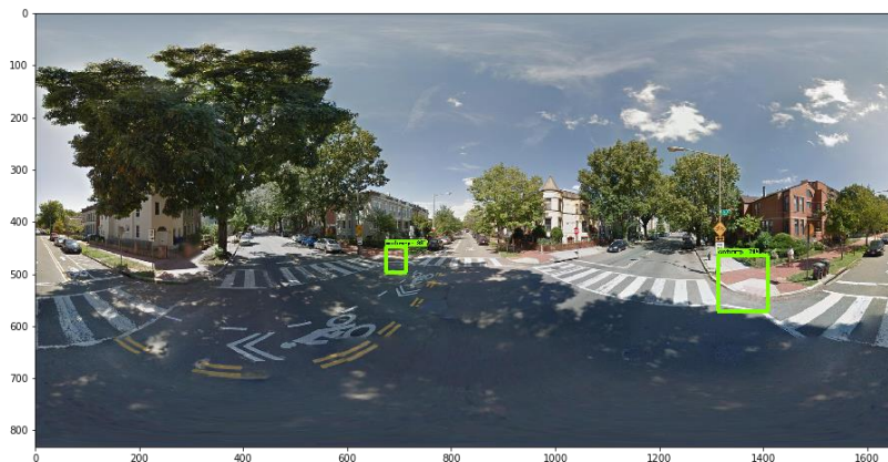
Figure 3. Example of model output showing correct detection of curb ramps.
