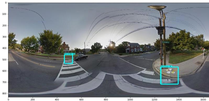
**Figure 3.** Example of model output showing correct detection of curb ramps.
