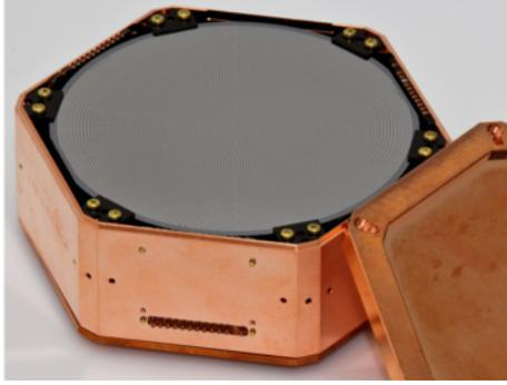
(a) Photo of a SNOLAB HV detector in its copper housing. The face of the detector looks different than the iZIP detectors because there are no charge electrodes interleaved between the phonon TESs. There will be germanium and silicon versions of this detector.
