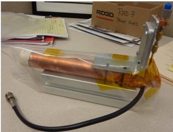
(a) Pictured is the prototype ULBPC used for most of the measurements shown here. There was a small leak, so the end of the tube was dipped in TorrSeal, which led to the prototype getting its nickname “Marshmallow.” It does not have the block of copper shielding that new ULBPCs are made with, so it is essentially just an electroformed copper tube strapped to a piece of aluminum framing.
