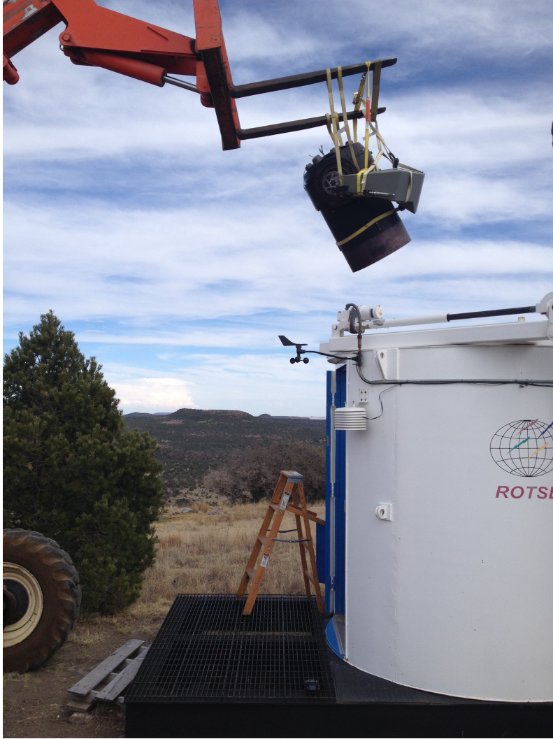
Figure 2.5: Removal of the ROTSE OTA from the enclosure. This removal was necessary to facilitate the refurbishments needed to return ROTSE-IIIb to on sky observing.
