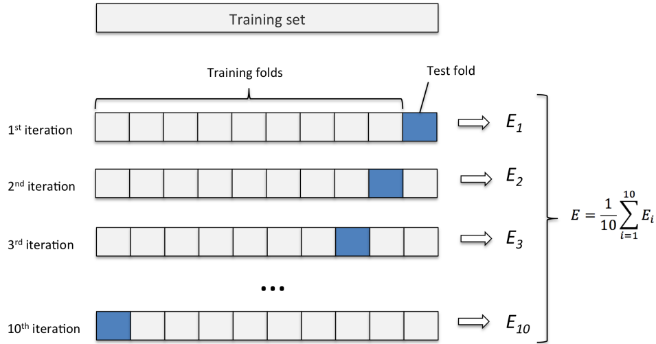
Figure 2.10. 10 fold cross validation, reported performance are averaged across 10 folds. Image source from [4].
