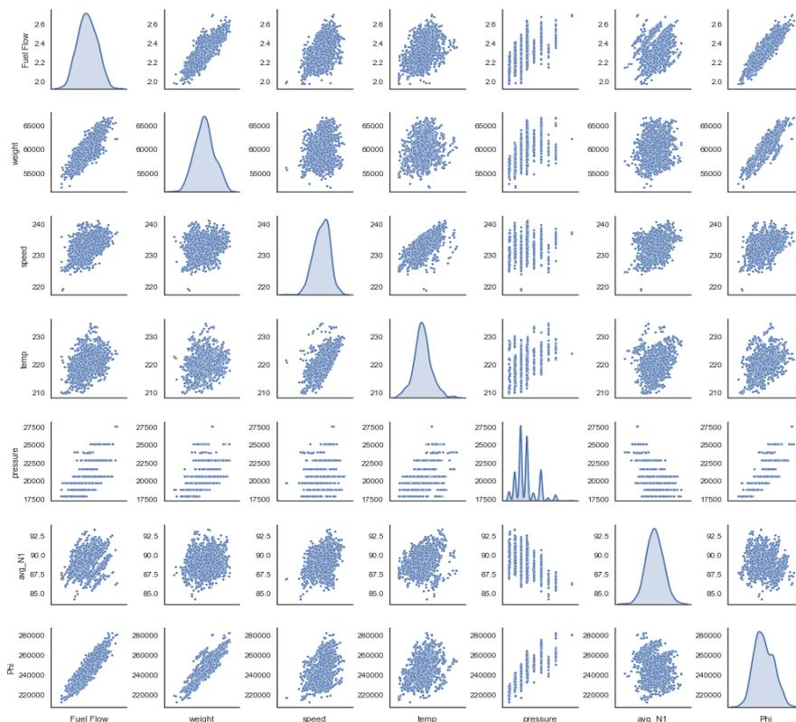
**Fig. 1.** Matrix of scatter plots for most of the relevant features used in the analysis. Most have very normal distributions and are linearly proportional to fuel flow.
