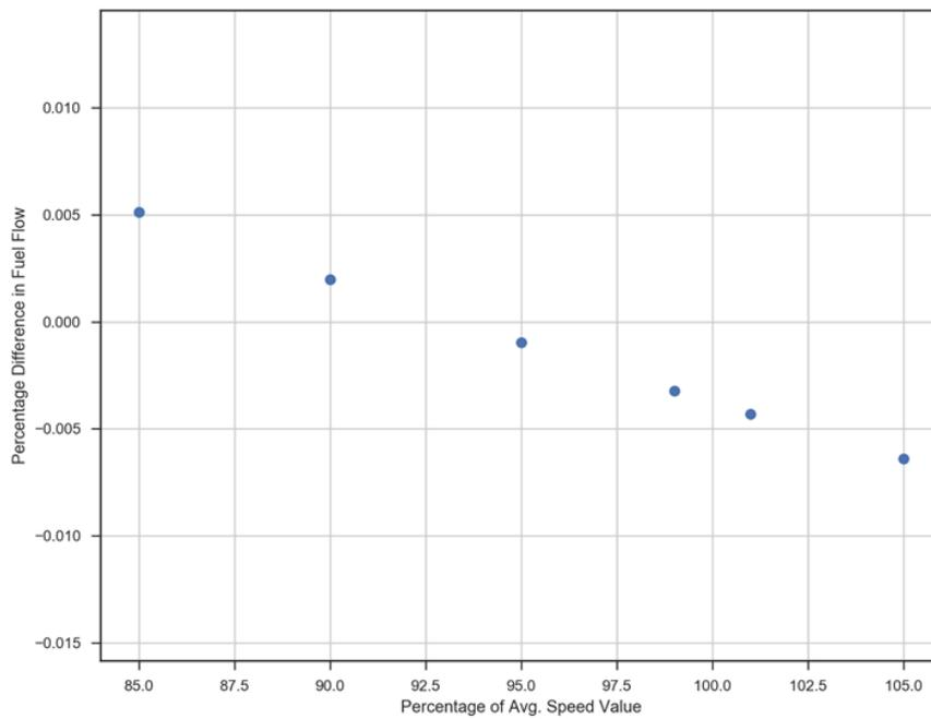
**Fig. 7.** Changes in fuel flow for different values of speed. This shows improved efficiency in fuel flow with smaller values speed for AC-001.
