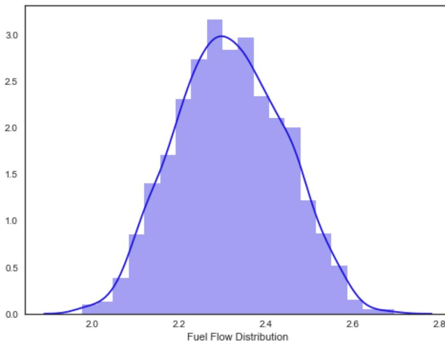
**Fig. 2.** The distribution of Fuel Flow from flight steady state data for three-minute sliding windows. This shows that Fuel Flow has a normal distribution for three-minute sliding windows for numerous flights after application of the CVG product.
