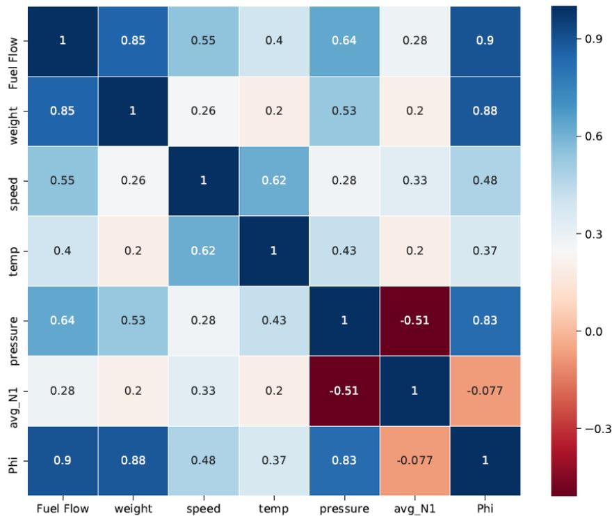
**Fig. 4.** Correlation coefficients of selected features. The function Phi has a high correlation with Weight, Pressure, and Fuel flow.
