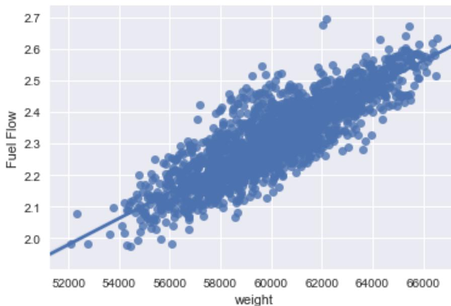
**Fig. 3.** The Fuel Flow is plotted versus the weight of AC-001. This graph clearly shows the linear nature of the relationship between the weight of the aircraft and the fuel flow.
