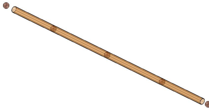
Fig. 4.2 Sketch of test channel (heated section) with flowing particles
