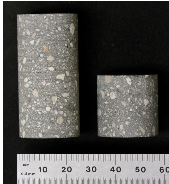
Fig. 14. Pristine cylindrical BBR9 high-strength concrete specimens with L/D = 2.0 (left) and L/D = 1.0 (right)
