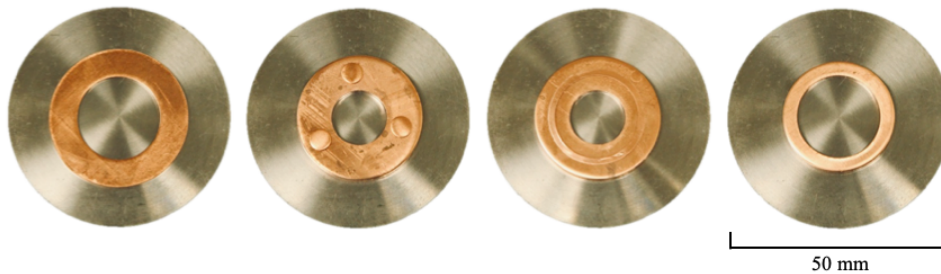
Fig. 40. Pulse shapers for confinement pressures of (left to right) 10 MPa, 50 MPa, 100 MPa, and 200 MPa.
