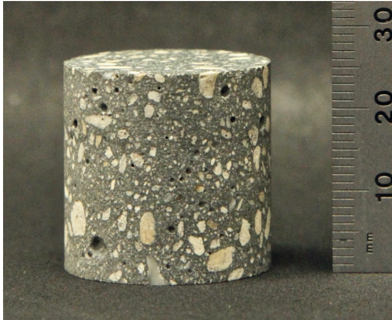
Fig. 34. Cylindrical BBR9 high-strength concrete specimen.
