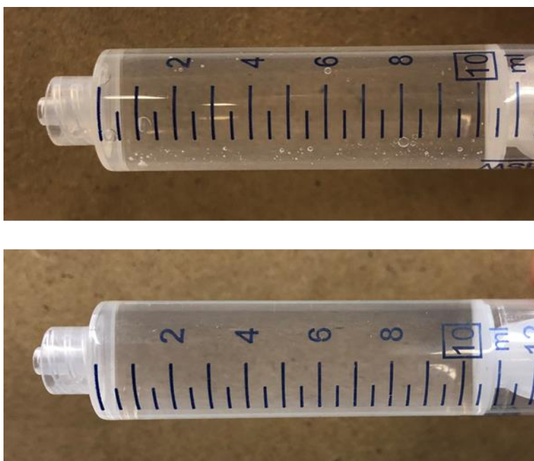
Figure 6 Syringe and liquid with no deaeration (top) and syringe with deaeration (bottom).
