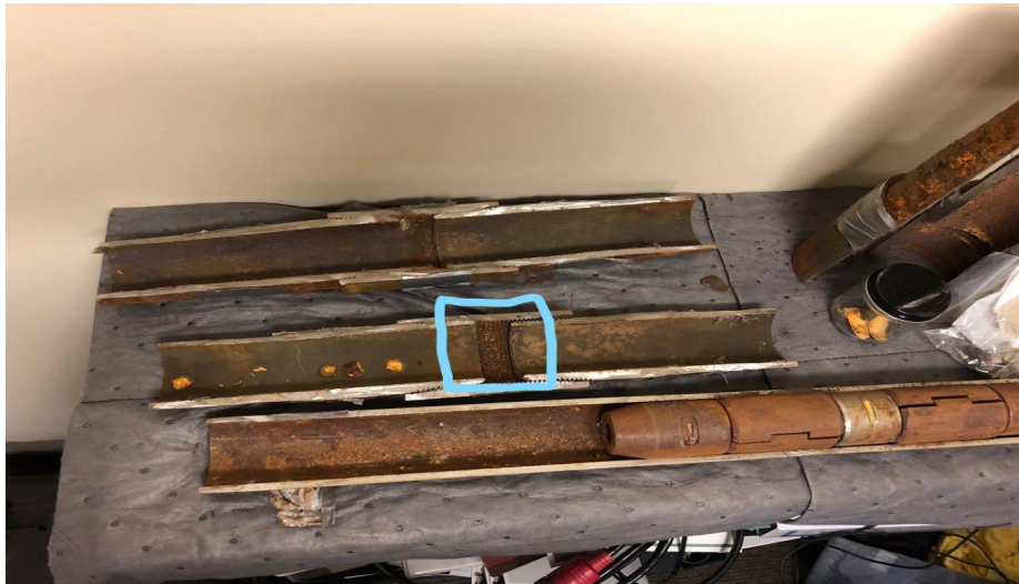
Fig. 2. Example of a natural gas well collar joint (highlighted in blue). Picture by Atsu Atakpa, 2018.
