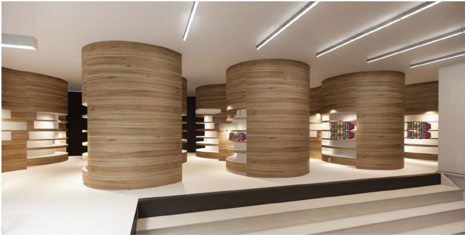
Stacks Perspective Rendering. The lighting in the room follows the structure of the book stacks. The flow and shape of stacks simulates a topography of mountains and enhances the experience of being in the middle of a mountain range. The LED strip light used along the perimeter of each shelf serves as ambient, task, and wayfinding.
