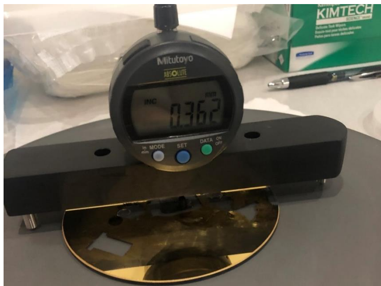
Figure 108. Measuring the wafer thickness using a digital thickness gauge
