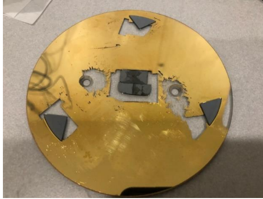
Figure 109. Wafer and dummy pieces waxed on top of the chuck facing down.
