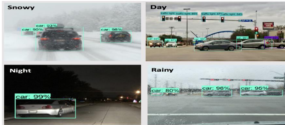
Fig. 2. Object detection under four different driving conditions: Snowy, Day, Night and Rainy.
