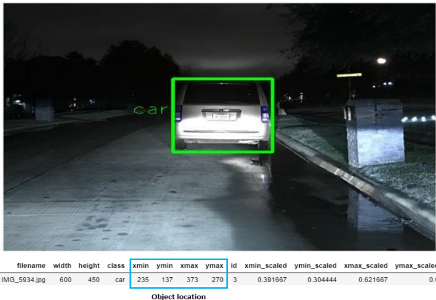
Fig. 18. Sample ground-truth info for the location of a car in an image.
