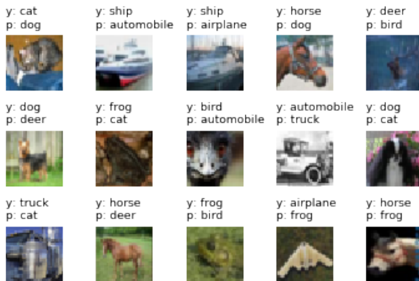
Fig. 9. Misclassified image samples by the basic CNN model M0. The upper panel y is to show the ground truth image and the lower panel p is to show the corresponding predicted image. This image misclassification is caused by model overfitting.
