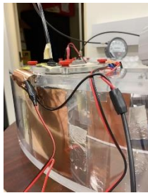
Figure 10: Field source alternating signal copper foil setup
