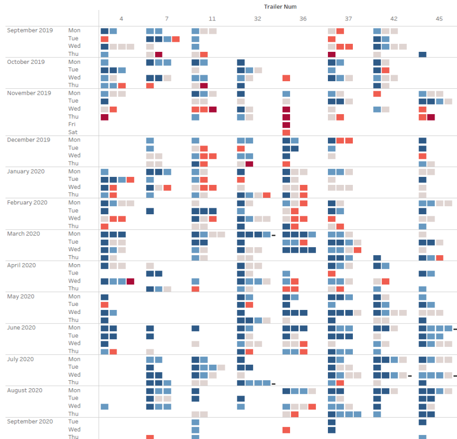
Fig. 1. Trailer utilization by day of week. Of note is how most of the trailers were not going out full. The redder the square, the less optimized it is for that day of the week. In this visualization we can see the trends clearly to lead us down the next path in the data.
