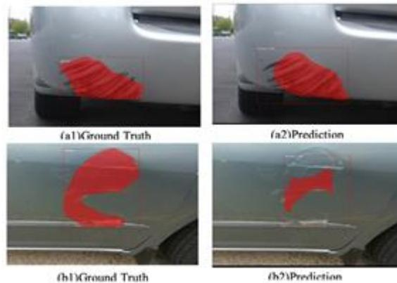
Fig. 9. (a1) Car Damage Ground Truth label with image 1 (a2) Car Damage prediction with image 1. (b1) Car Damage Ground Truth label with image 2 (b2) Car Damage prediction with image 2.
