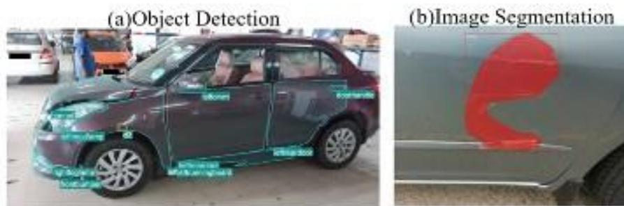
**Fig.1. (a)** Example image with car parts detection **(b)** Example image with damage area segmentation
