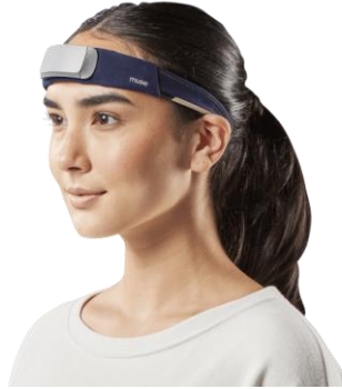
Fig. 1. Muse headset, a wearable EEG device used for brainwave data collection, equipped with four EEG electrodes strategically positioned at TP9, AF7, AF8, and TP10 locations on the scalp
