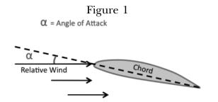
Exceeding the critical angle of attack causes the airflow around the wing to separate and create such an excess of drag over lift that the wing can no longer function to keep the airplane on the desired flight path. The result is a loss of control if
