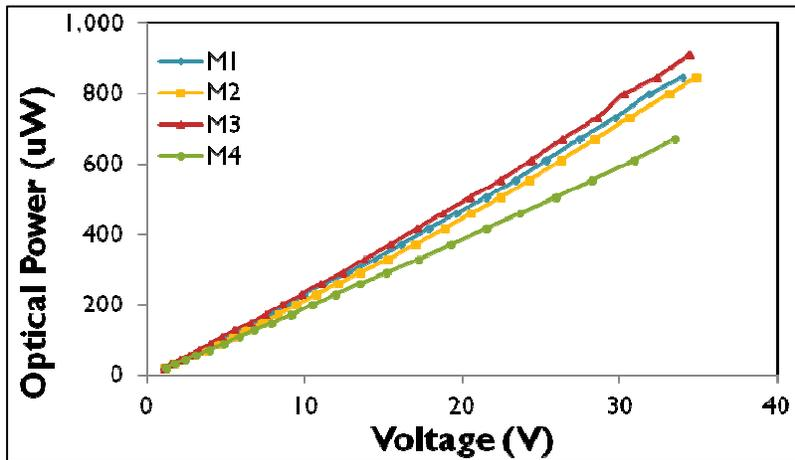
Figure 8. Power-voltage curves for each fiber
